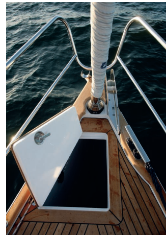
With no fairlead from bow roller to cleat, she needs a deck windlass
