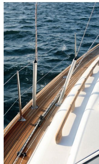
Moving forward is easy, with great toerails and grabrails
