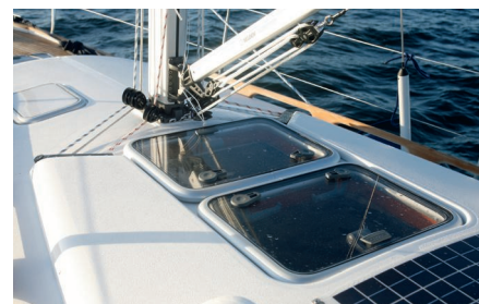
The flush Lewmar hatches light up the saloon and ventilate well
